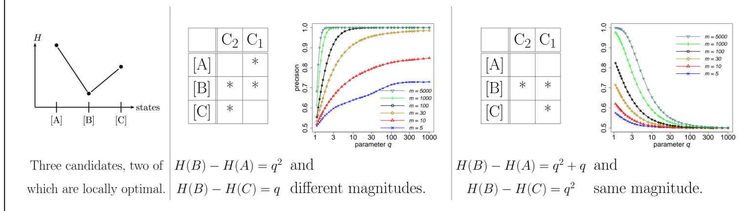
**Precision of simulated annealing** with different cooling schedules, as a function of q
